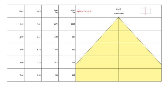
Note: In case of lighting fixture with more than one lighting source, the illuminance plane is referred to the single lighting source.
