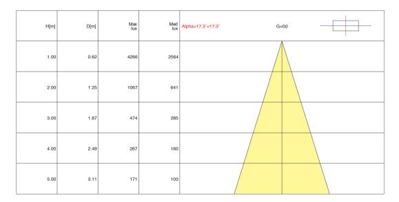
Note: In case of lighting fixture with more than one lighting source, the illuminance plane is referred to the single lighting source.
